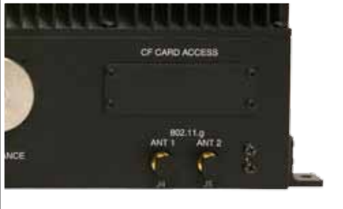
An 802.11G Wireless Access Point connects passenger laptops and wireless cabin phones.
